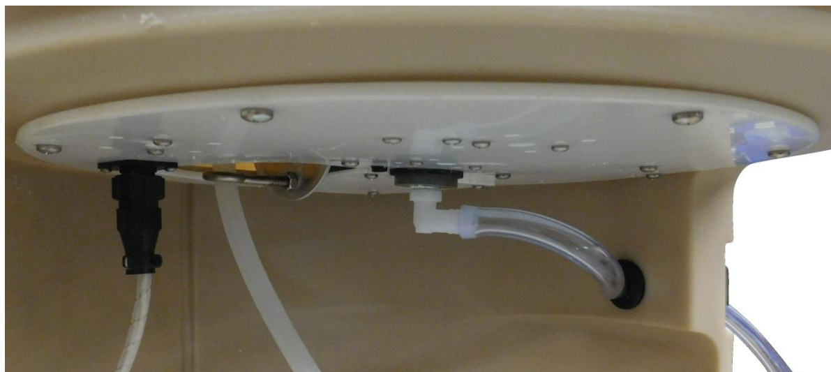
Figure 2-1: Connect Intake Line to Sample Chamber Intake Riser
