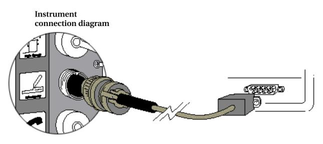
Direct connections -2100 and Field Wizard A USB RS-232 Communications Cable, Isco P/N 60-2004-507, connects the 2100 Series instrument to your PC's USB port. An RS-232 Communications Cable, Isco P/N 60-2004-046, connects the 2100 Series instrument to your PC's Com port. Refer to the diagram below.
