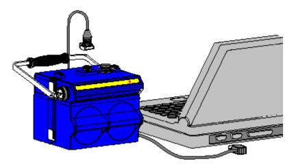
The 2101 Field Wizard does not have a case top connector. Instead, the communications cable attaches to the connector on the right side of the case.
