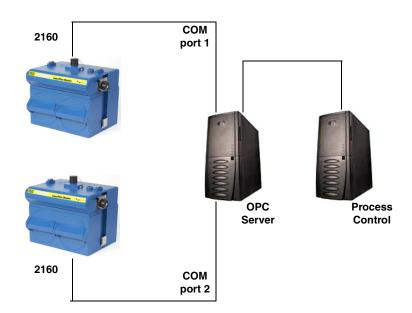
Figure 4-1 Configuration example
