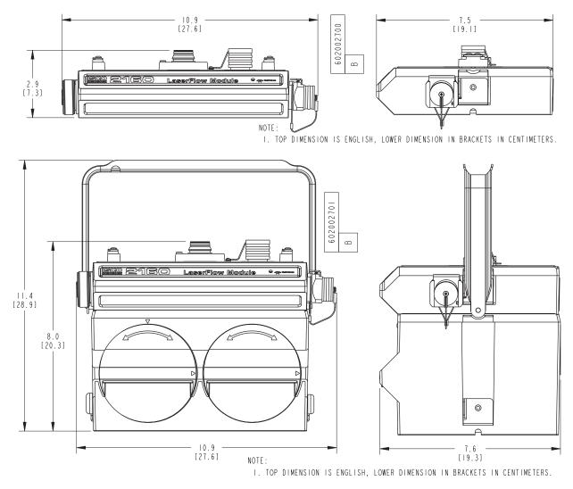
Figure 1-6 2160 LaserFlow Module dimensions: Alone (top) and with 2191 Battery Module (bottom)
