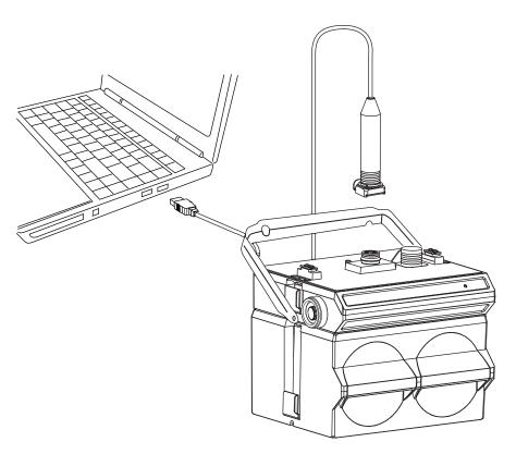
Figure 3-1 Connecting the 2160 to a computer
