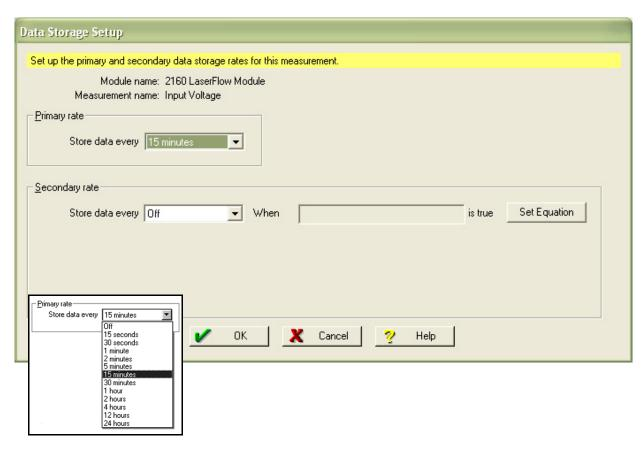
Figure 3-3 Data Storage Setup in Flowlink
