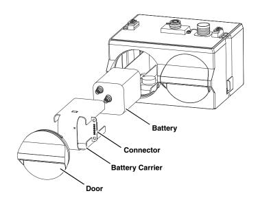
Figure 1-3 2191 Battery Module key components
