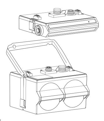
Figure 2-2 Align and secure the module stack
