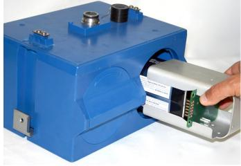
2. Insert the carrier and battery into the module. Note the position of the carrier's connector; it must be aligned toward the center of the module.
