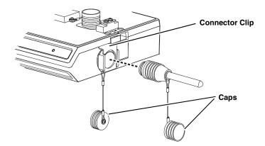
Figure 2-3 Connecting the LaserFlow sensor
