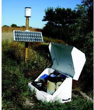
The 2105 system shown here interfaces with a rain gauge, flow meters, automatic sampling, and a multi-parameter sonde.
