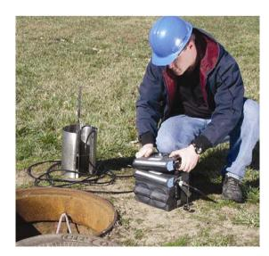
The 2150EX is approved to the ATEX Directive 94/9/EC by Baseefa, and to Class I, Division 1 by CSA for use in manholes and other hazardous locations. A second flow module can be stacked to provide redundant or multistream measurement.
