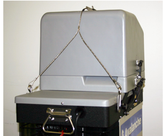
Figure 8: Y-cable across controller top cover
