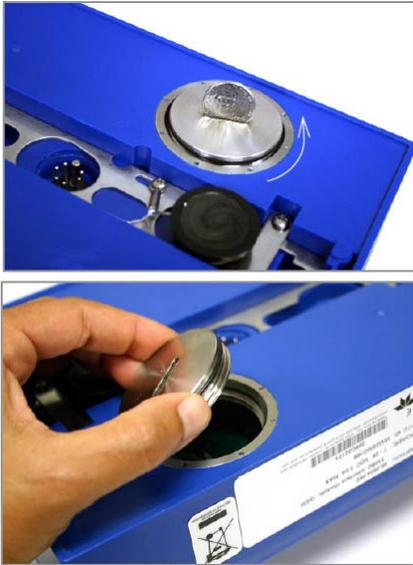
**Figure 3: Removing the SIM cover**
