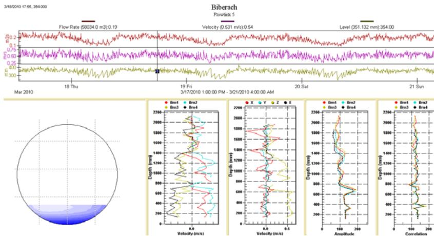
Measurement results displayed in Flowlink 5.1 software, with flow profile and velocity diagnostics. Lower velocities in profile shown in darker color.
