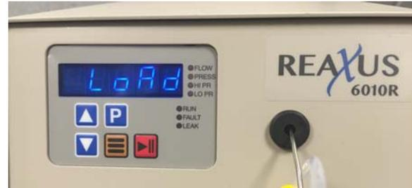
**Figure 3: ReaXus pump screen in firmware update mode**
