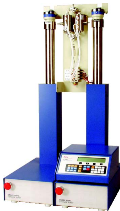
Figure 3: Dual pump system for continuous flow (A500HLf with air valves shown)
