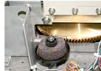
**Figure 5: Lube wheel** (Saturate with ALMASOL 609)
