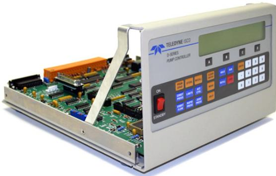
**Figure 1: Flat panel controller** Part #60-5364-388
