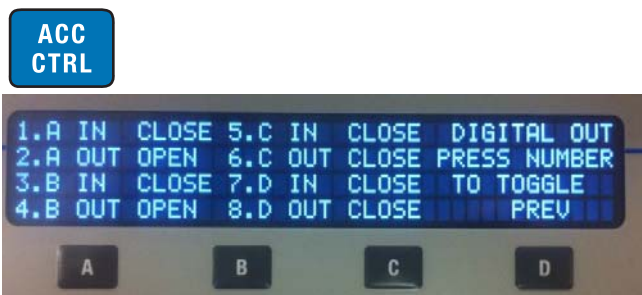
Figure 9: Using accessory control menu to test valves for proper connection
