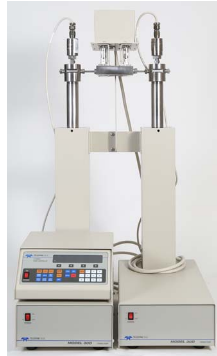
Figure 1: 30D system with electric valves
