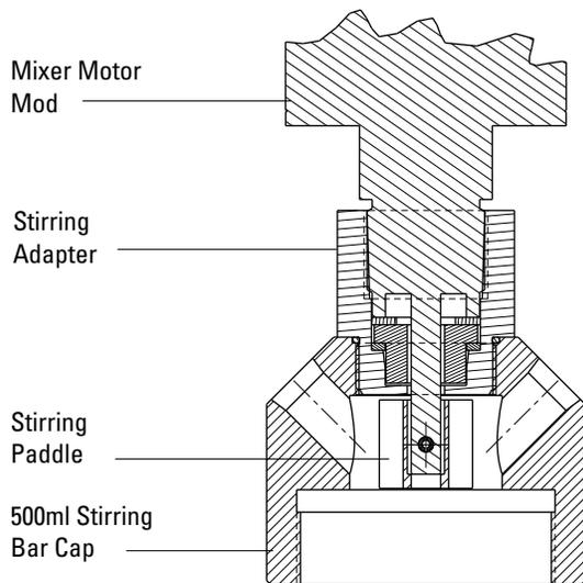
**Figure 1: Syringe pump stirring cap**
