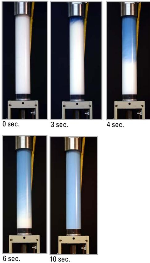
**Figure 4: Distribution time: Blue dye + 20% w-w cornstarch slurry**
