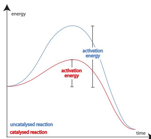
**Figure 2: Boltzman Energy Diagram for reaction pathway**
