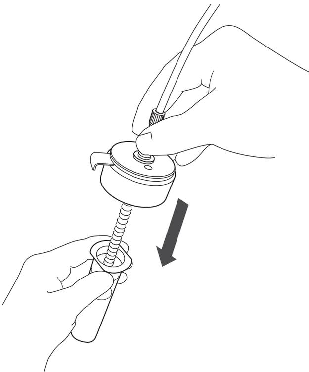
**Figure 3: Insert the plunger to the bed**
