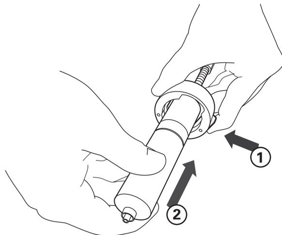
**Figure 4: Align and push cartridge into the cap**
