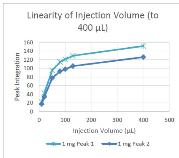
**Figure 2: Peak integration across multiple, different injection volumes for 100  $\mu$ L loop**
