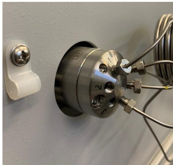
Figure 1 Original Uncoated Stainless-Steel stator installed in the ACCQPrep
