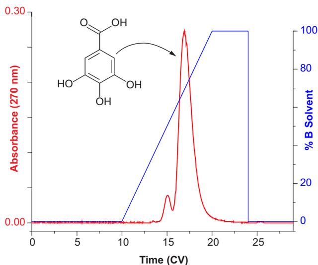
**Figure 1: Purification of Gallic Acid on a RediSep Rf SAX column**
