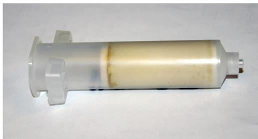
**Figure 4: RediSep C18 solid load cartridge "catches" retained compounds extending the life of the main C18 column**
