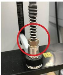
3. Connect the tube connected to the Torrent and the now free nut and ferrule and connect to the Union attached to the pre-swaged tubing.
