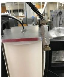
4. Remove the swaged plug from the top of the column with a wrench and replace with the tubing that is now connected via union to the Torrent.
