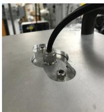
5. Remove the swaged plug from the bottom of the column with a wrench and replace it with the second piece of tubing that came with the column.
