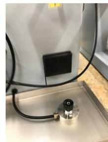
6. Remove the black fitting on the bottom port of the Torrent and connect the tubing from the bottom of the column to this port with the black nut.
