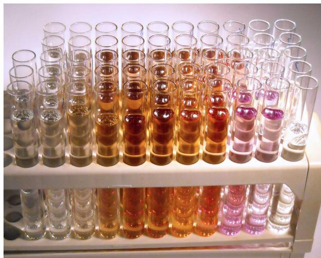
**Figure 2: Fractions on right exhibited the characteristic purple color of purified C<sub>60</sub> fullerene**
