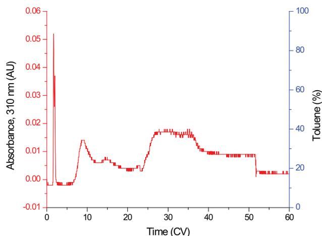
**Figure 1: Purification of C<sub>60</sub> using an Rf-200 flash system and RediSep Gold C18 column**
