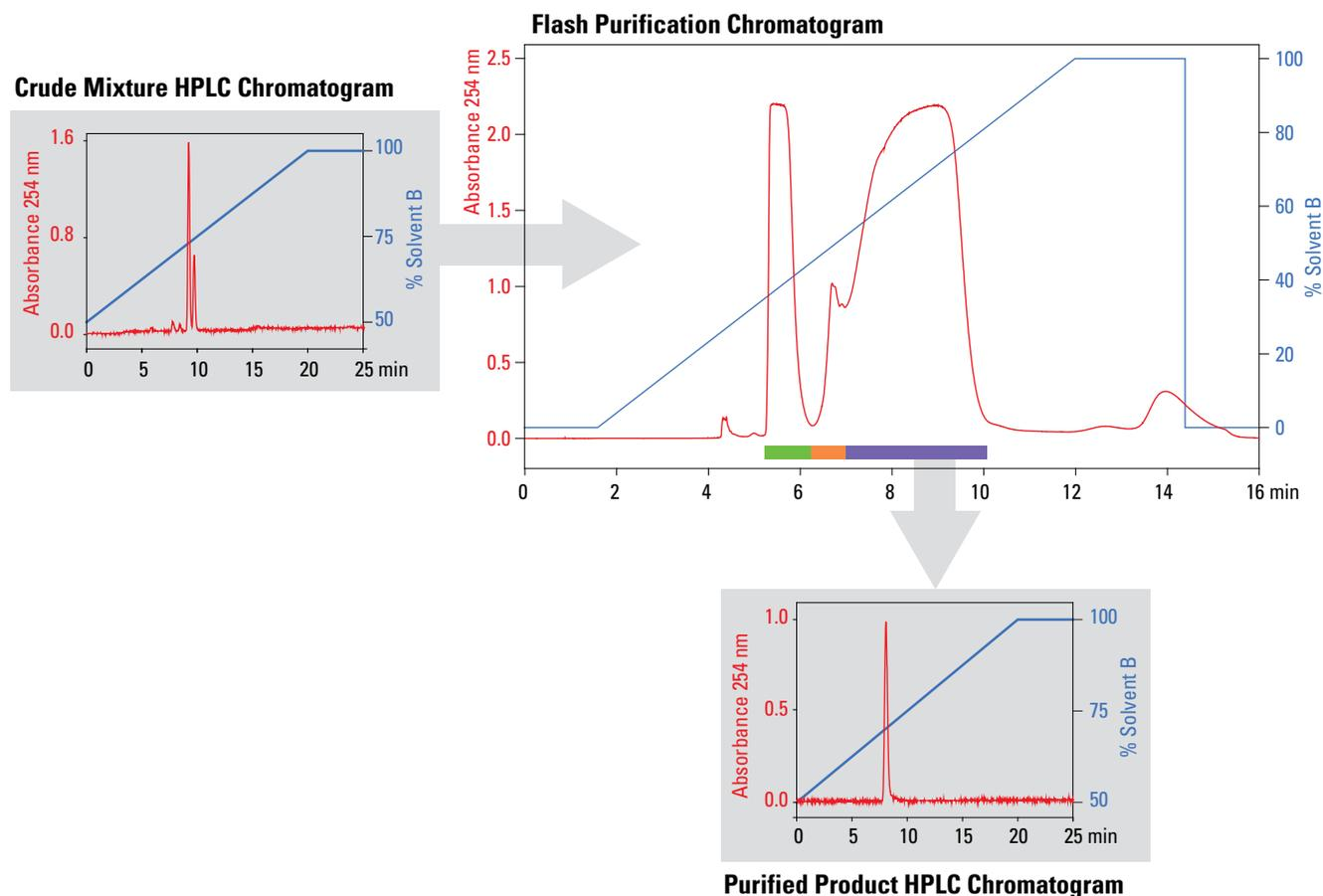
**Figure 2: Purification of 3-(2-nitrophenyl amino) propionitrile** using a CombiFlash Torrent, RediSep Rf 3 kg silica column, and 750 g solid load cartridge. HPLC chromatograms indicate purity of crude and purified product.
