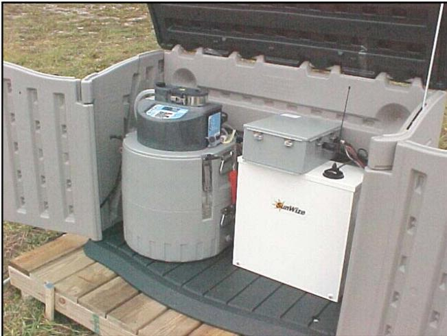
Challenges presented by the airport monitoring sites include the absence of telephone lines and AC power. These challenges were met by using cellular telephones for remote communication with the samplers, and a deep cycle battery and solar charger capable of powering the system with complete independence from utility lines.
