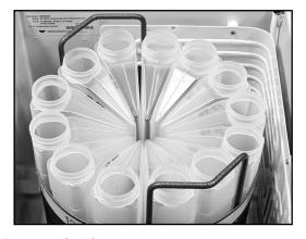
Figure 2-5 14-Bottle configuration completed
