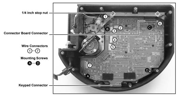
Figure 9-7 Main Circuit Board Connections
