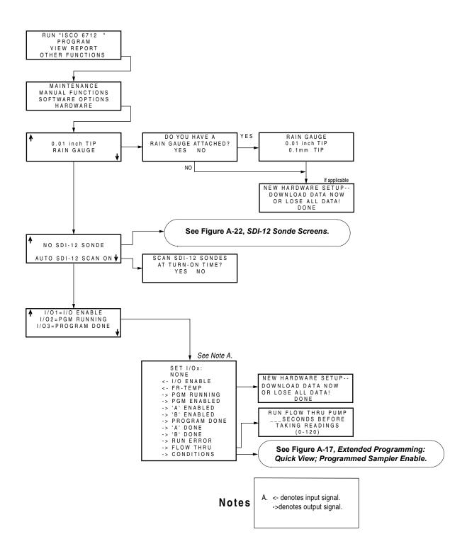
Figure A-21 Extended Programming: Quick View; Hardware
