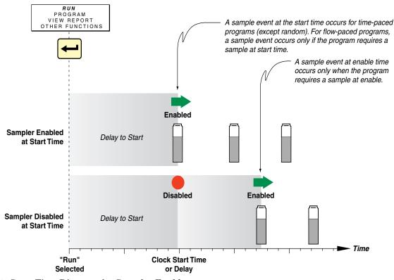
Figure 5-4 Start Time Diagram for Sampler Enable Settings
