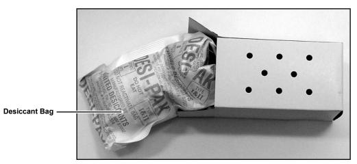
Figure 9-6 Removing the desiccant bag
