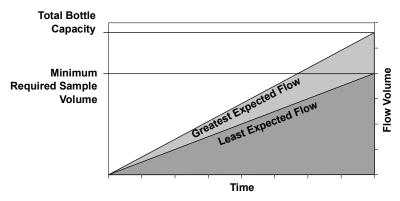
Figure 5-2 Factors affecting flow-weighted variable-volume samples
