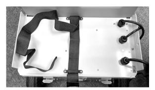
Figure 2-17Battery box strap installed
