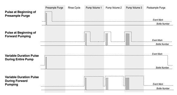
This diagram shows the pulses sent for a bottles-per-sample distribution scheme
