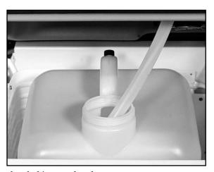
Figure 2-15 Composite 5 gallon bottle kit completed
