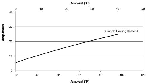
Figure F-1 Amp-hours required to cool 6 liters of sample liquid from 20 °C (A<sub>c</sub>)
