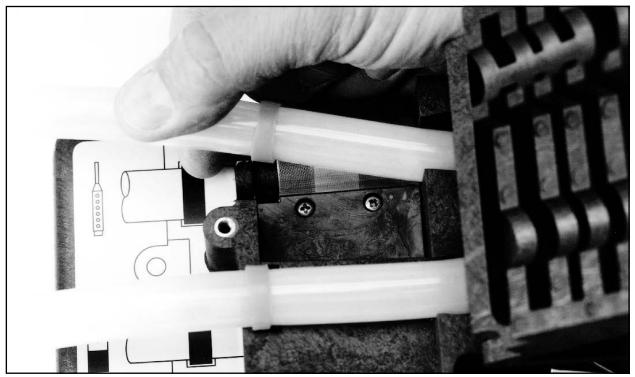
Figure 9-3 Placing the pump tube in the liquid detector
