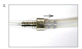
Figure 2-19 Attaching the suction line to the pump tubing
