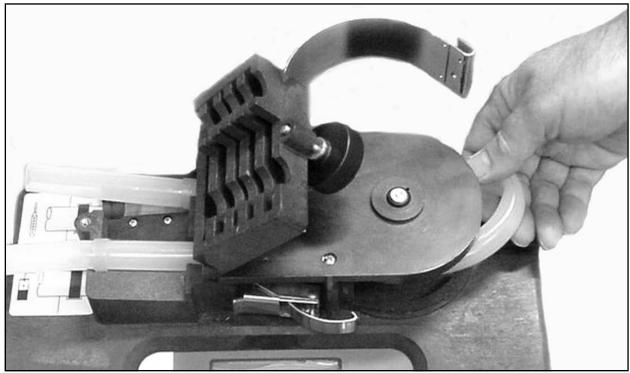
Figure 9-2 Removing and replacing the pump tube
