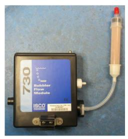
Figure 2-20 Desiccant cartridge and module.
