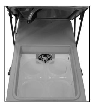
$Figure\ 2\text{-}8\ \ 4\text{-}Bottle\ configuration\ completed$
