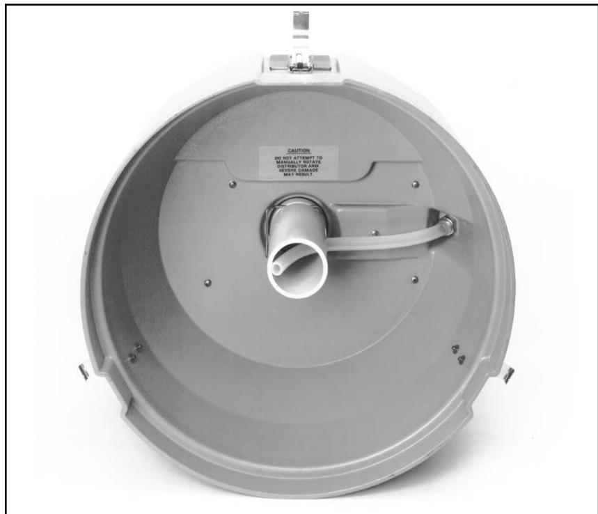
Figure 2-7 Installing the Composite Tube Guide
