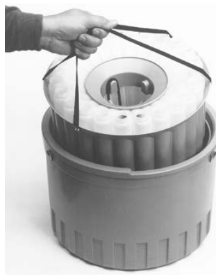
Removing Bottles From the Compact Sampler
