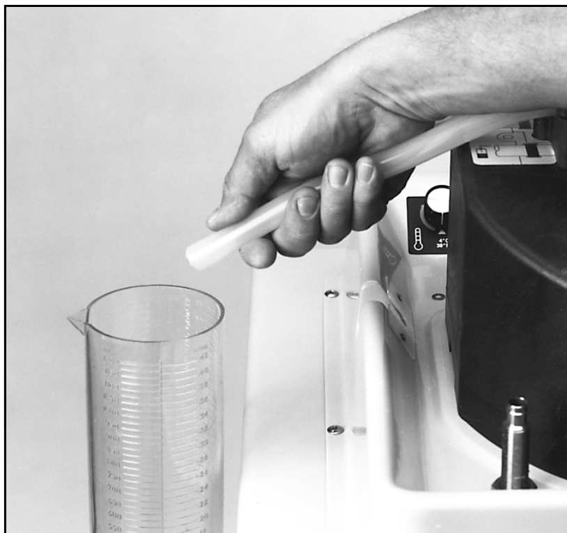
Figure 12 Taking a grab sample
