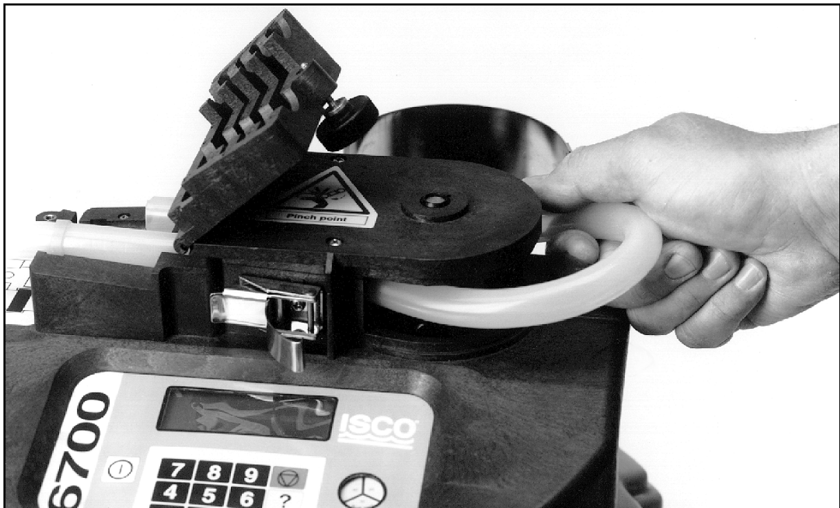
Figure 13 Removing and replacing the pump tube
