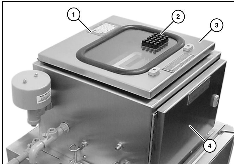
Figure 1-9 View of the purged enclosure and the access doors
