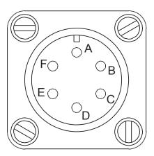
Figure 4-2 6-pin Connector Diagram
