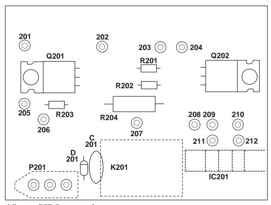
Figure 6-7 Optical Counter PCB Component Layout
