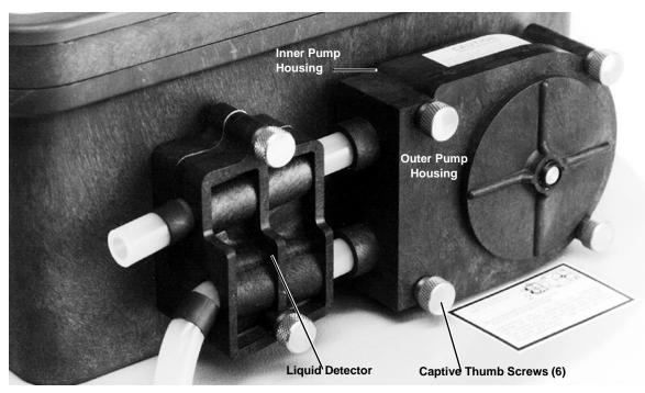
Figure 5-2 Liquid Detector and Pump Housing
