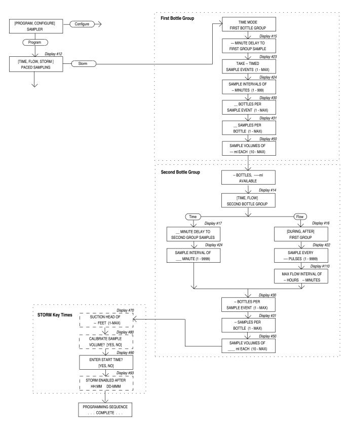
Figure 3-12 Extended Programming Mode: STORM Programming
