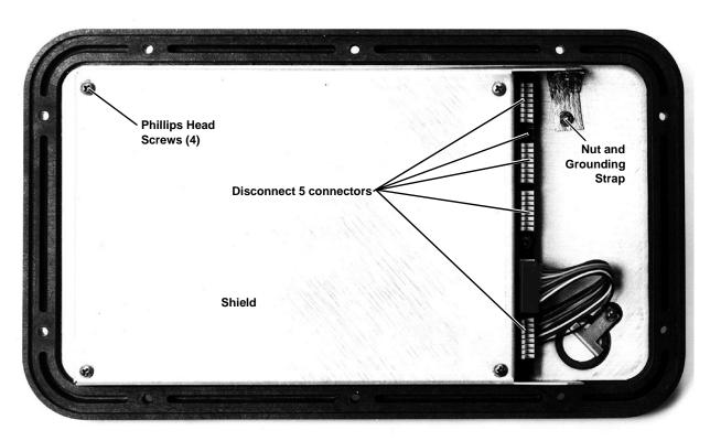
Figure 6-2 Underside of the Control Box Cover
