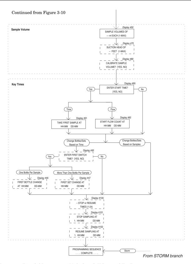
Figure 3-11 Extended Programming Mode: Sample Volume and Key Times
