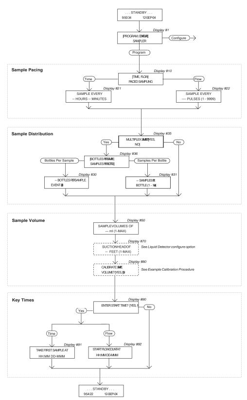
Figure 3-8 Basic Programming Mode: Program Sequence Structure
