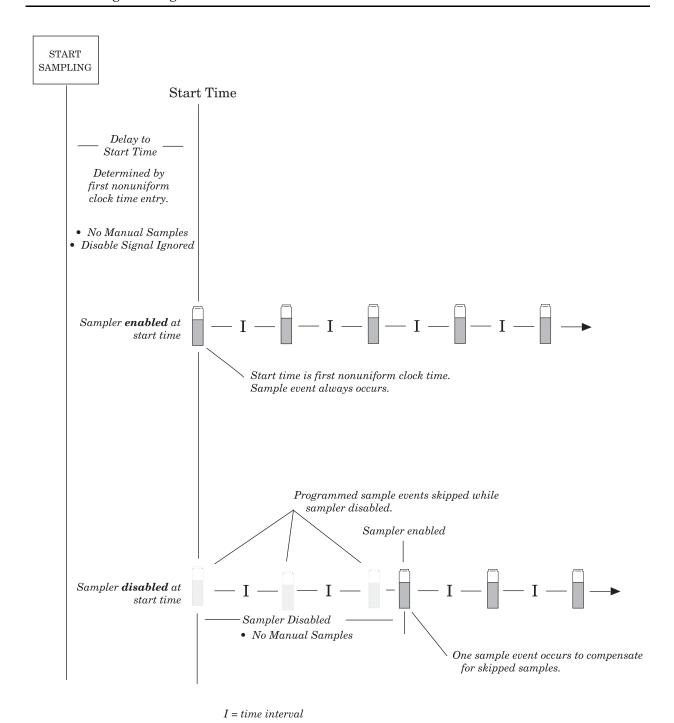
Figure 3-15 Start Time Diagram for Nonuniform Time Routines
