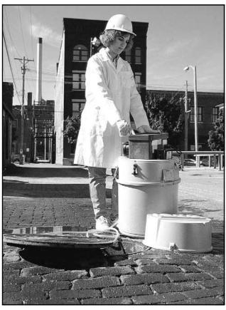
Figure 2-5 Placement of the Sampler Adjacent to Manhole
