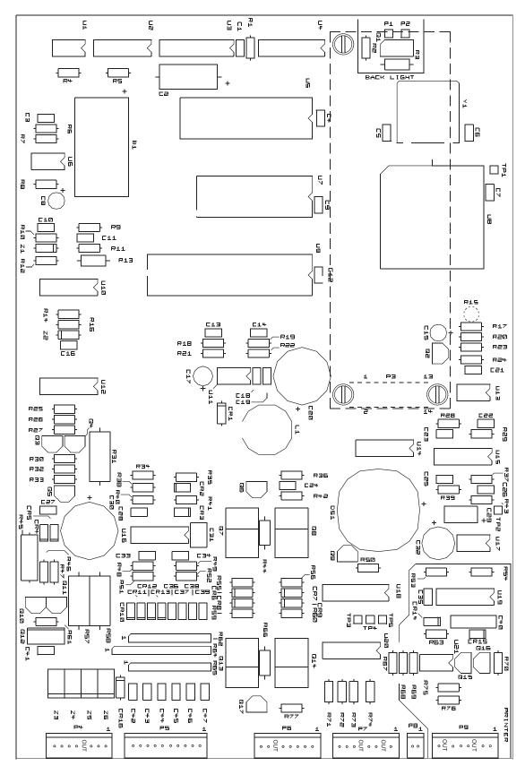
Figure 6-6 Main Circuit Board Component Layout
