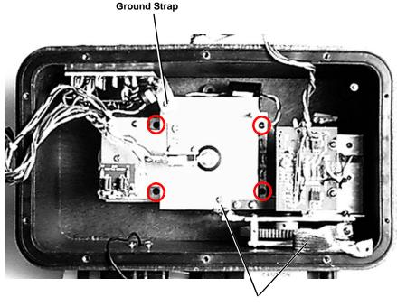
Unscrew the four screws and the ground straps to remove the distributor gear case.
