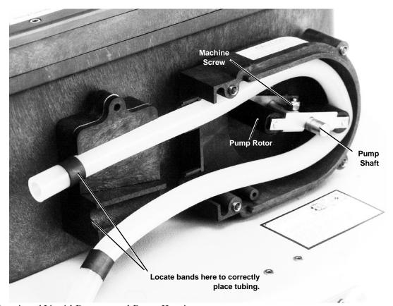
Figure 5-3 Interior of Liquid Detector and Pump Housing
