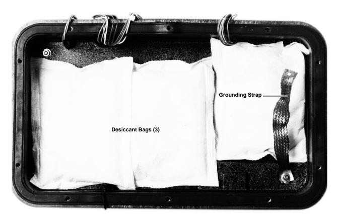
Figure 5-5 Internal Desiccant (controller lid removed)
