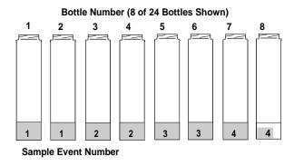
Figure 3-3 Bottles-Per-Sample Multiplexing
