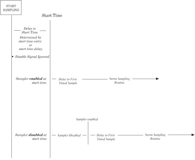
Figure 3-18 Start Time Diagram for STORM Routines
