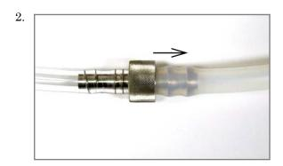
Figure 2-1 Attaching the suction line to the pump tubing
