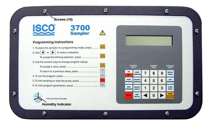
Figure 5-4 Location of 10 Screws on Control Box Lid
