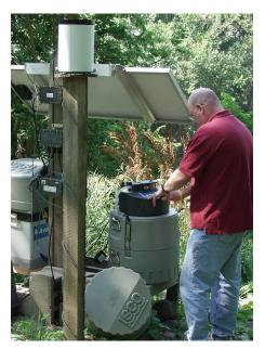
The CDMA cellular phone modem works with 6700 Series samplers, and the Avalanche® Portable Refrigerated Sampler. A rain gauge, 700 Series Flow Module, and/or SDI 12 multi-parameter sonde can be connected to the sampler for integrated monitoring. Data logged by the controller can be downloaded via the modem.
