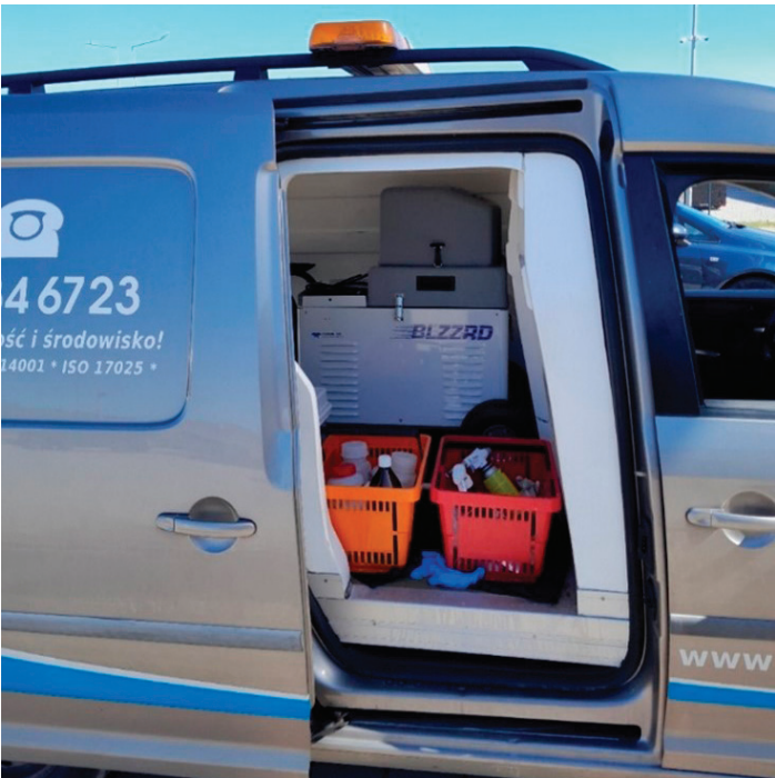
The BLZZRD sampler is transported to sites by van and usually left there for one day. After samples are collected, they are sent to the accredited laboratory for analysis of specific parameters required by the discharge permit authorization.
