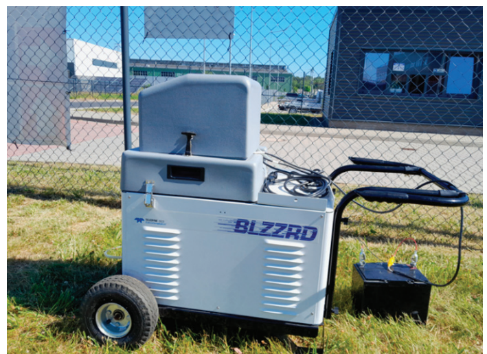
Battery powered BLZZRD portable refrigerated sampler
