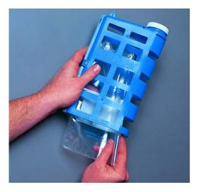
1,000 ml ProPak bags install quickly into light-weight, reusable holders. A 2-gallon capacity bag is also offered for composite sampling.
