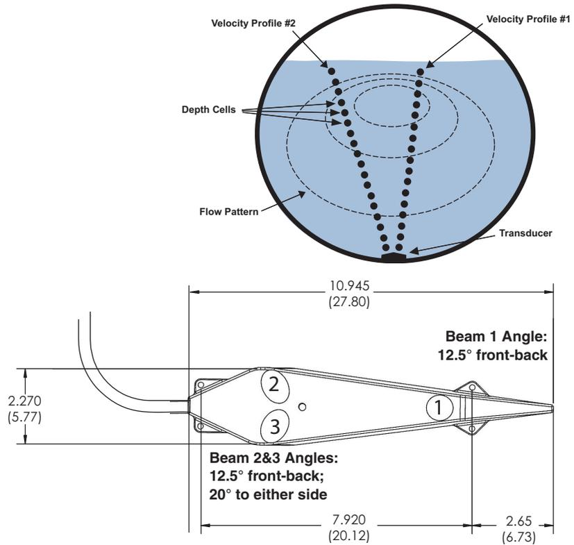
Figure 1-2 Pulse Doppler flow measurement, dimensions, and beam angles
