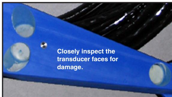
Figure 1-3 accQmin sensor inspection
