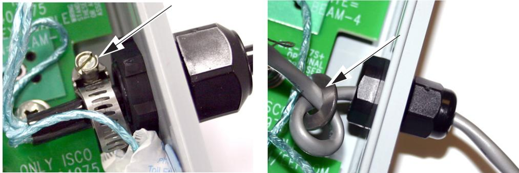
Figure 3-10 Strain relief for sensor extension cables
