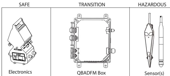
Figure 3-1 accQmin IS system components
