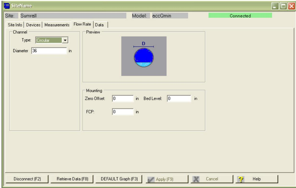
Figure 2-4 Flowlink Flow Rate tab: Circular channel
