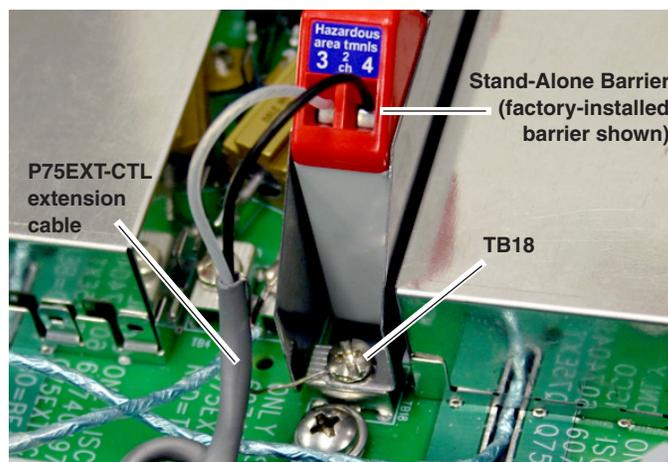
Figure 3-9 Disconnecting the secondary level sensor extension cable
