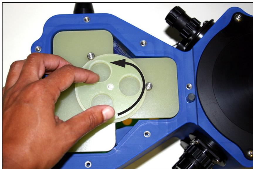
Figure 4-3 Loosening the battery retaining plate assembly
