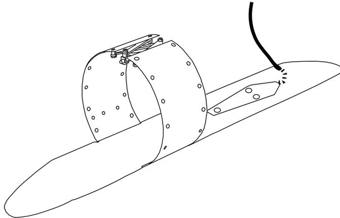
Figure 2-21 Sensor installation with FCP and scissors ring
