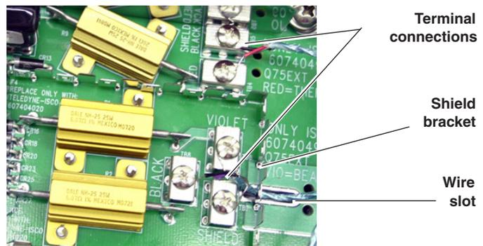
Figure 3-7 Wire routing and connections
