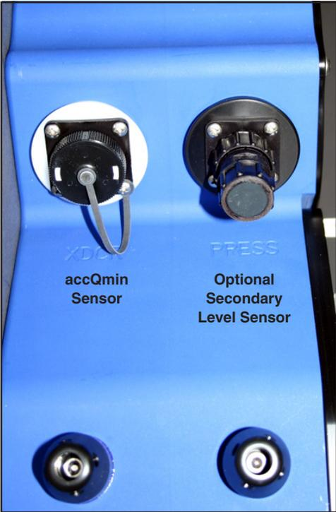
Figure 1-4 accQmin connections, left side
