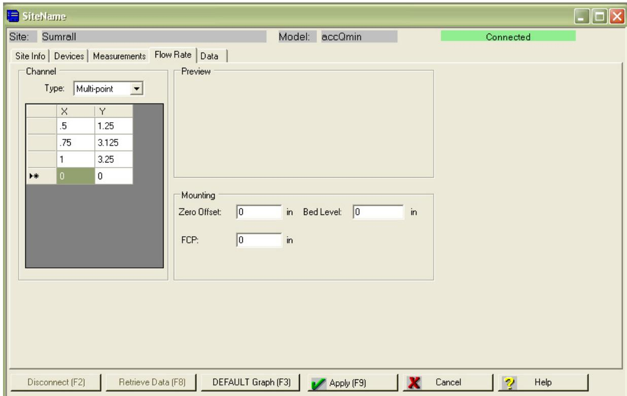
Figure 2-5 Flowlink Flow Rate tab: Multi-point channels
