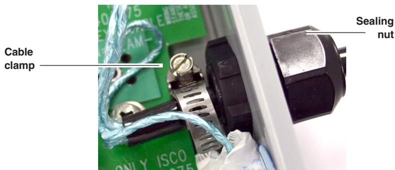
Figure 3-8 Release cable from clamp and cord-grip fitting
