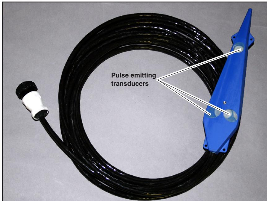
Figure 1-1 accQmin velocity sensor
