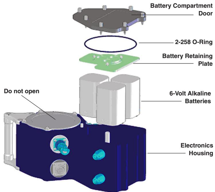
Figure 4-1 Battery replacement
