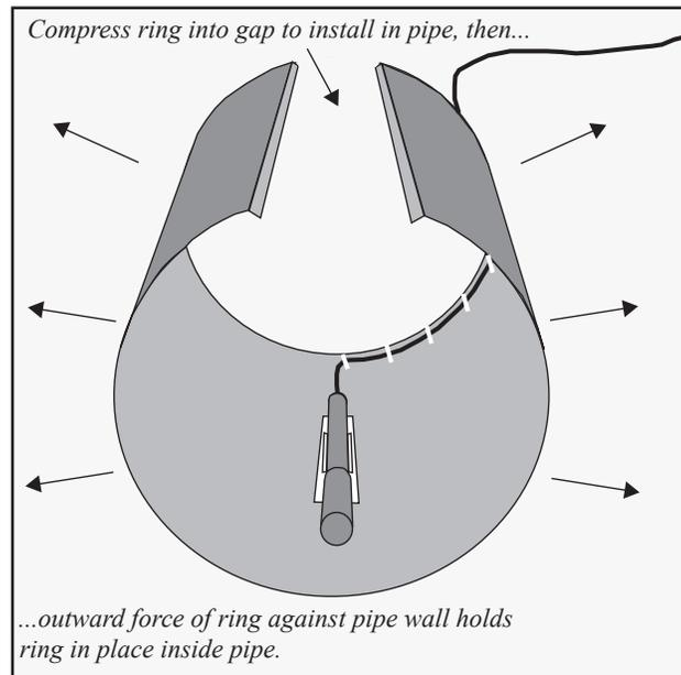
Figure 2-19 Sensor Installed on a Spring Ring
