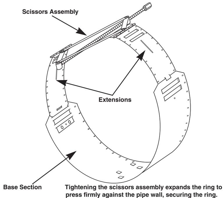
Figure 2-20 Scissors Ring adjustment
