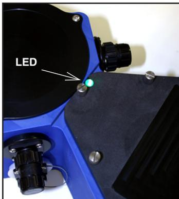
The housing contains an LED indicator that shows the operational status of the accQmin. Different combinations of color and state indicate the data quality, deployment status, and connector port status. Table 1-1 lists the possible status conditions indicated by the various states and colors of the LED indicator.
