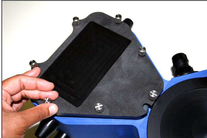
Figure 4-2 Battery cover removal
