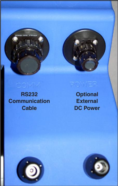
Figure 1-5 accQmin connections, right side
