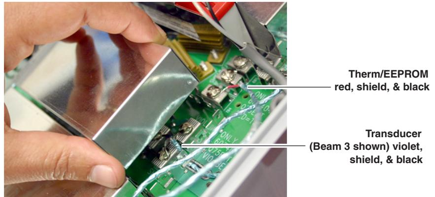
Figure 3-6 Accessing accQmin thermal and transducer terminal connections
