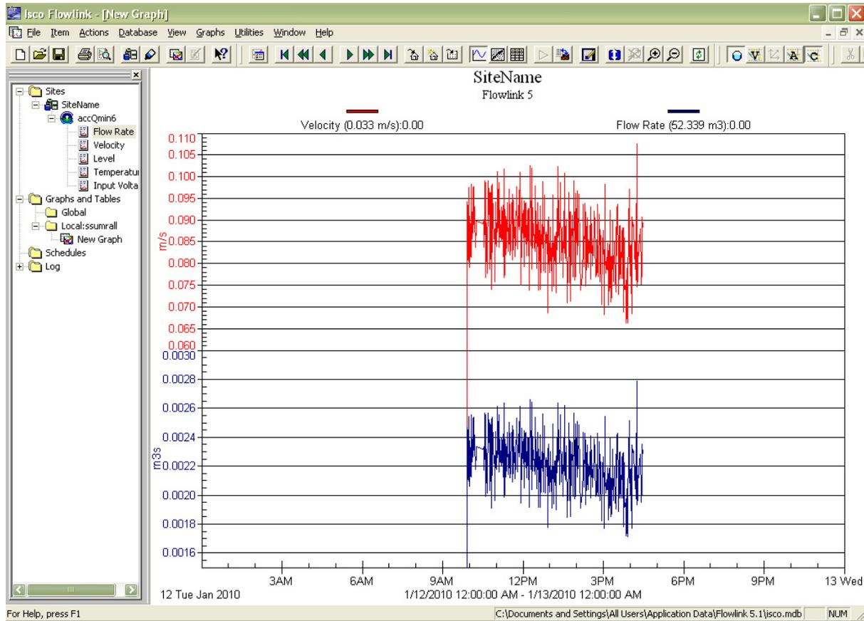
Figure 2-29 Flowlink: Drag & drop data parameters on graph (velocity and flow shown)
