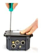
Figure 5-3 Remove the 6 screws
