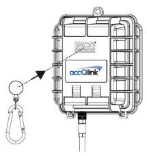
Figure 2-2 Turing on the accQlink device using the activator
