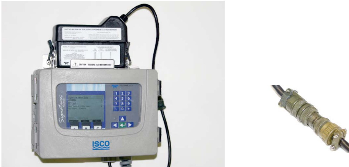
Figure 5-8 Backup battery, installed
