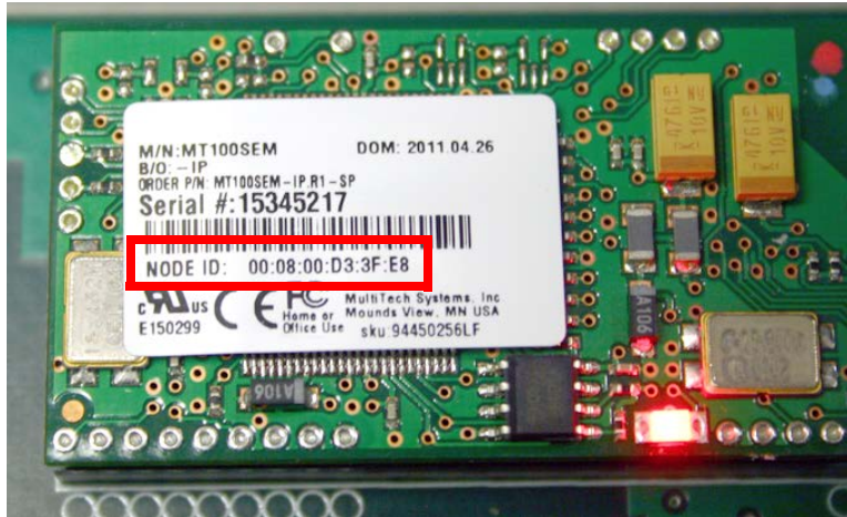
Figure 5-31 Locating the NODE ID (MAC address) on the ethernet modem
