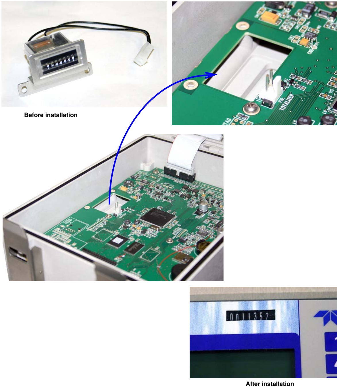
Figure 5-10 Optional non-resettable totalizer installation
