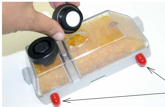
Figure 6-8 Opening the desiccant cartridge chambers
