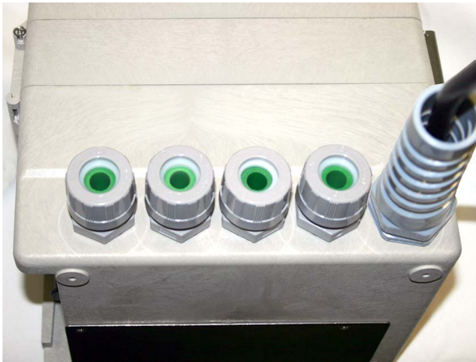
Figure 3-5 Cord-grip fittings installed
