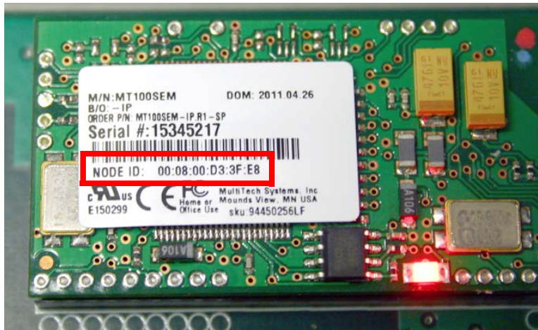
Figure 5-35 Locating the NODE ID (MAC address) on the ethernet modem
