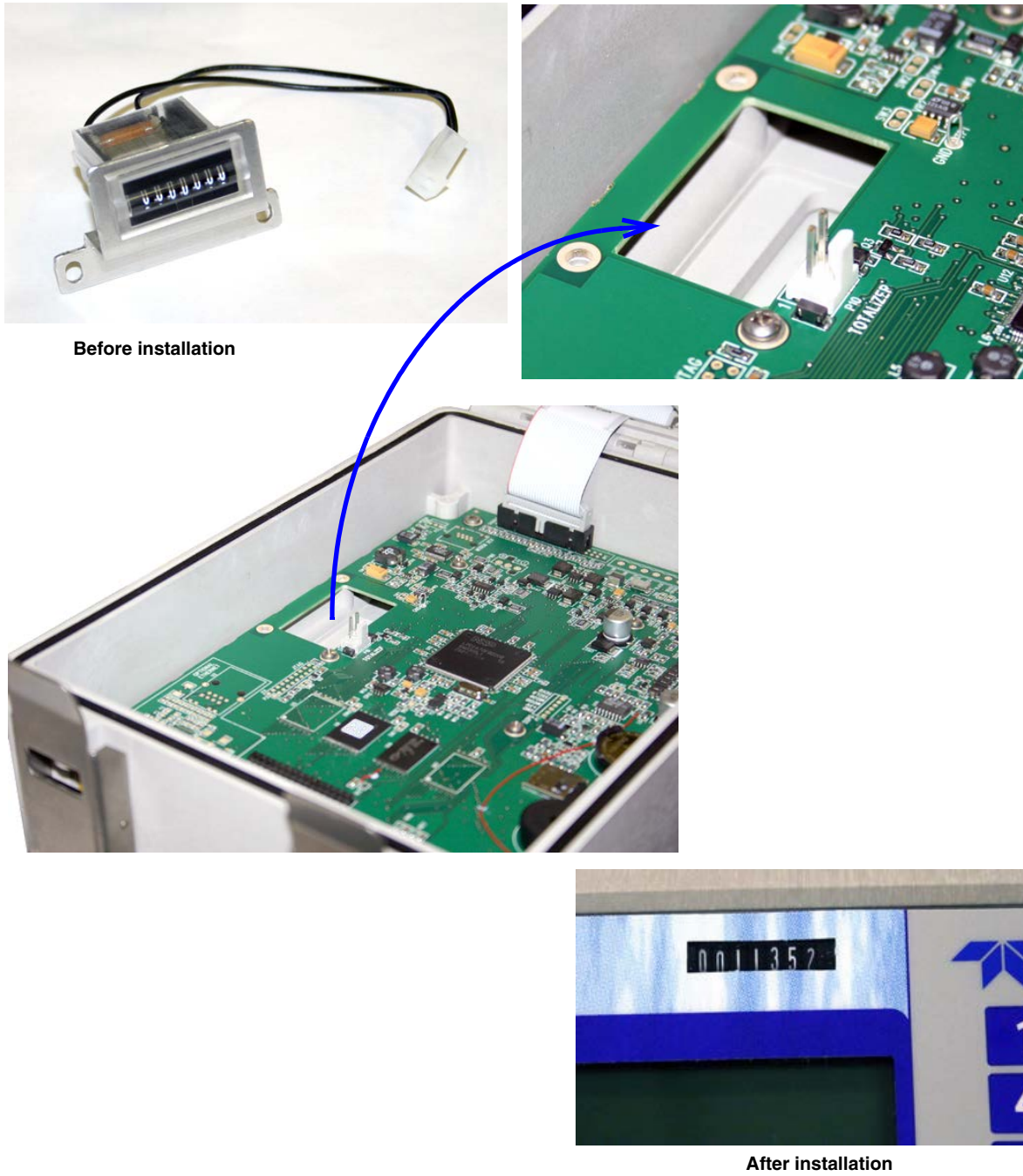
Figure 5-11 Optional non-resettable totalizer installation
