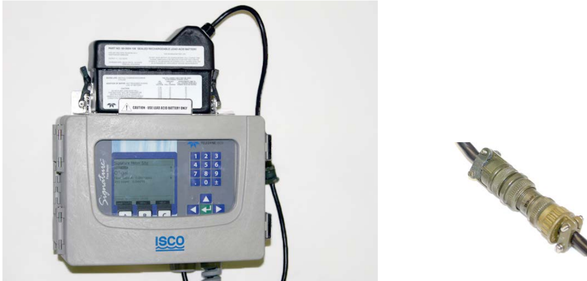
Figure 5-8 Backup battery, installed
