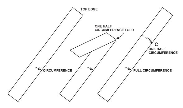
6) Once again, wrap the paper around the pipe starting with the top edge corner positioned at the second transducer location (separation distance point B).
