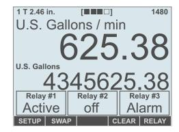
The flowmeter remains in the **Run Mode** until it is powered down, the user takes an action to go to Setup Mode or, exceptionally, an error occurs and the flowmeter goes to the **Faulted State**. The user can command the flowmeter to **Setup Mode** by pressing the motherboard setup button or changing the position of the measurement mode switch between Transit Time and Doppler.
