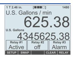
total volume of fluid flow. The flowmeter is not sensitive to the direction of fluid movement and *flow in either direction is treated as positive* for both flow rate display and accumulation of the total volume of fluid that has passed (totalization). Should fluid flow first in one direction and then return in the other direction, the flowmeter will register a total of twice the amount of fluid, even though the net actual flow is zero.
