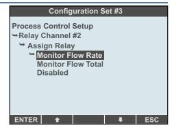
Under the **Process Control Setup** branch, sub-branches appear for each of the three Relay Channels.
