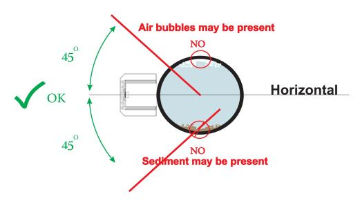
4.6 Doppler Method Transducer Installation
