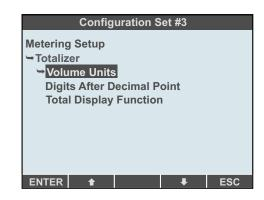
**Flow Total --> Total Display Function** allows you to enable or disable the clearing of the recorded total flow using the **CLEAR** soft button on the display in **Run Mode** and also the clearing of batch counts and totals on **Process Control Screens**.
