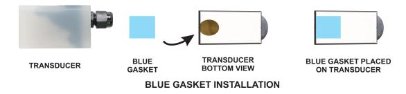
Dow Corning Silicone Seal #111 (part number 90008-394) may be used in place of the gaskets if desired.
