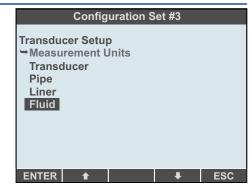
**Configuration Set** is "activated", but not when a user exits **Setup Mode** by "escaping" (for example, after the five minute timeout). Note that changes in this area of configuration followed by an escape from **Setup Mode** may cause the flowmeter to display incorrect flow information.
