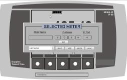
Press SAVE EDITS. The IP ADDRESS must match the IP address configured in the meter SPU. See section 5.2.1 of this manual. If the meter is installed on a network, the IP address must be an address that is available to the network. Contact your IT department for assistance with network configurations. The new meter can now be selected and activated.
