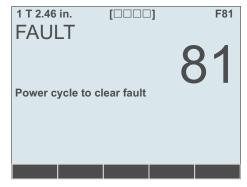
To exit the **Faulted state**, it is necessary to power cycle the flowmeter. If the error is due to configuration problems, these should be addressed before allowing the flowmeter to reenter the **Run Mode**, see section 7 below.
