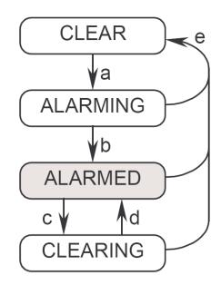
this state, the relay is not energized. The status displays as Status: **ALARMING** in alternating black-on white and white-on-black and the **CLEAR** soft button is present. If the **CLEAR** soft button is pressed, counting down the **Alarm Delay Time** restarts. This state gives an operator time to correct the condition causing the alarm or for the condition to correct itself if it is transient.
