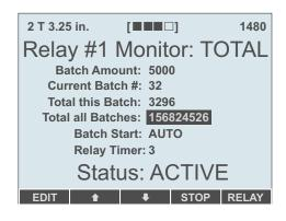
This continues indefinitely (unless the **STOP** soft button is pressed). Each time the **Total this Batch:** totalizer reaches **Batch Amount:**, it is cleared, **Current Batch #:** advances and the relay is energized for the time **Relay Timer:**.
