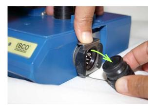
Figure 2-10 Preparing the 2160 connector receptacle
