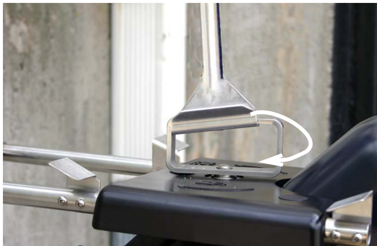
Figure 2-30 Turn the locking handle clockwise until sensor is locked into place (shown with the optional sensor retrieval arm, described in Section 2.8)
