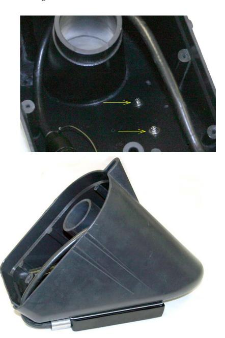
Figure 5-5 Mounting the integrated  $350\,\mathrm{AV}$  sensor on the LaserFlow
