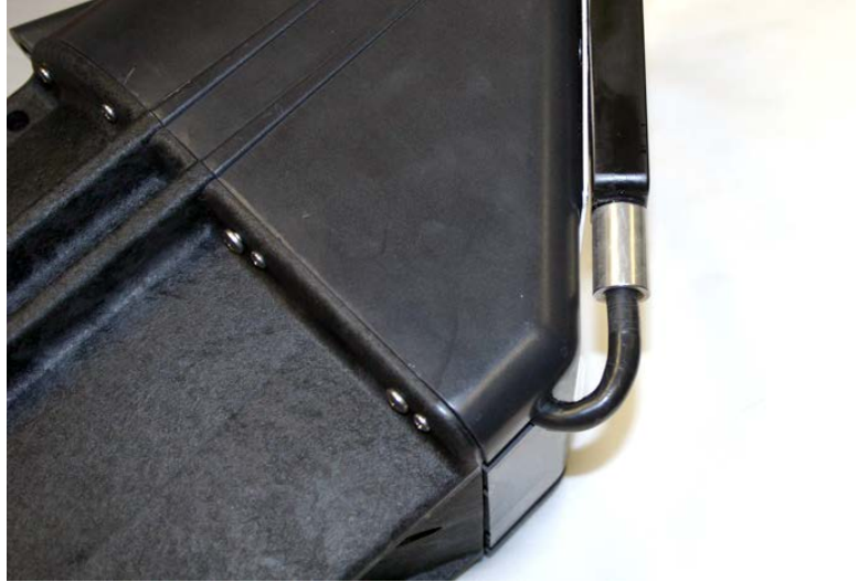
Figure 5-7 Reassembling the LaserFlow w/ AV sensor installed
