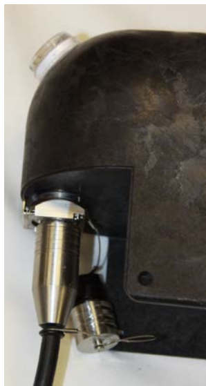
Figure 2-9 Secure caps and connect 310 ultrasonic plug to LaserFlow
