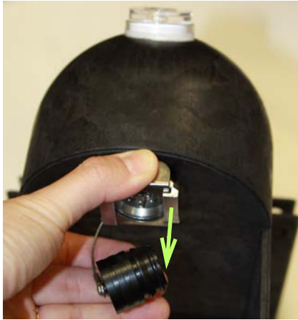
Figure 2-8 Preparing the LaserFlow connector receptacle
