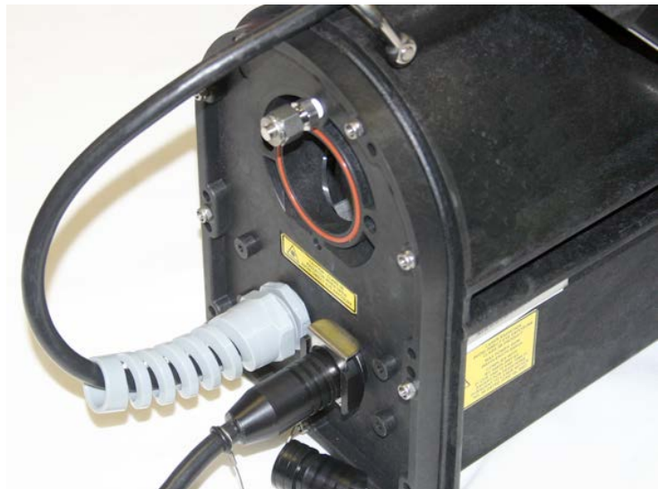
Figure 5-6 Connecting the 350 AV sensor to the LaserFlow
