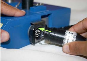
Figure 2-11 Secure caps and connect LaserFlow to 2160
