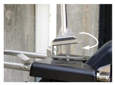
Figure 2-22 Turn the locking handle clockwise until sensor is locked into place (shown with optional sensor retrieval arm, described in Section 2.8)
