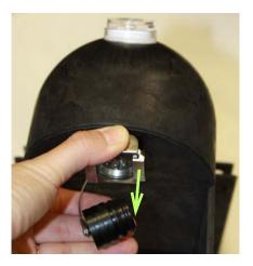
Figure 2-8 Preparing the LaserFlow connector receptacle
