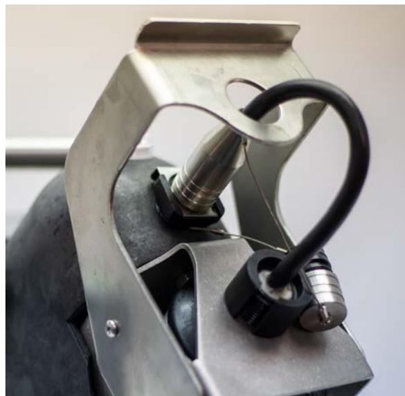
*Figure 2-13 Secure caps and connect the 310 ultrasonic
