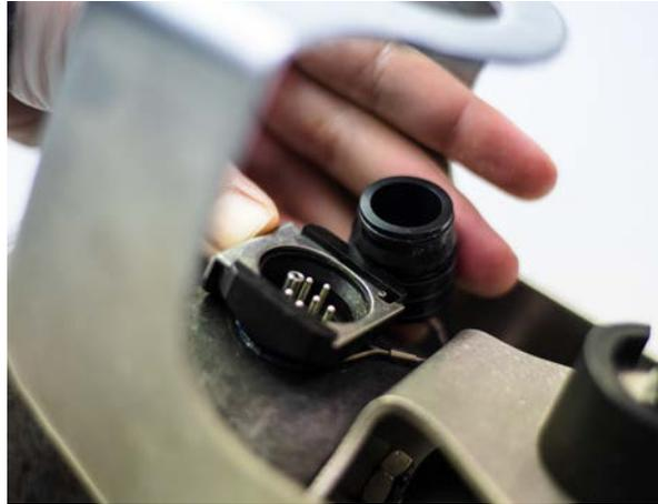
*Figure 2-12 Preparing the LaserFlow Ex connector receptacle*
