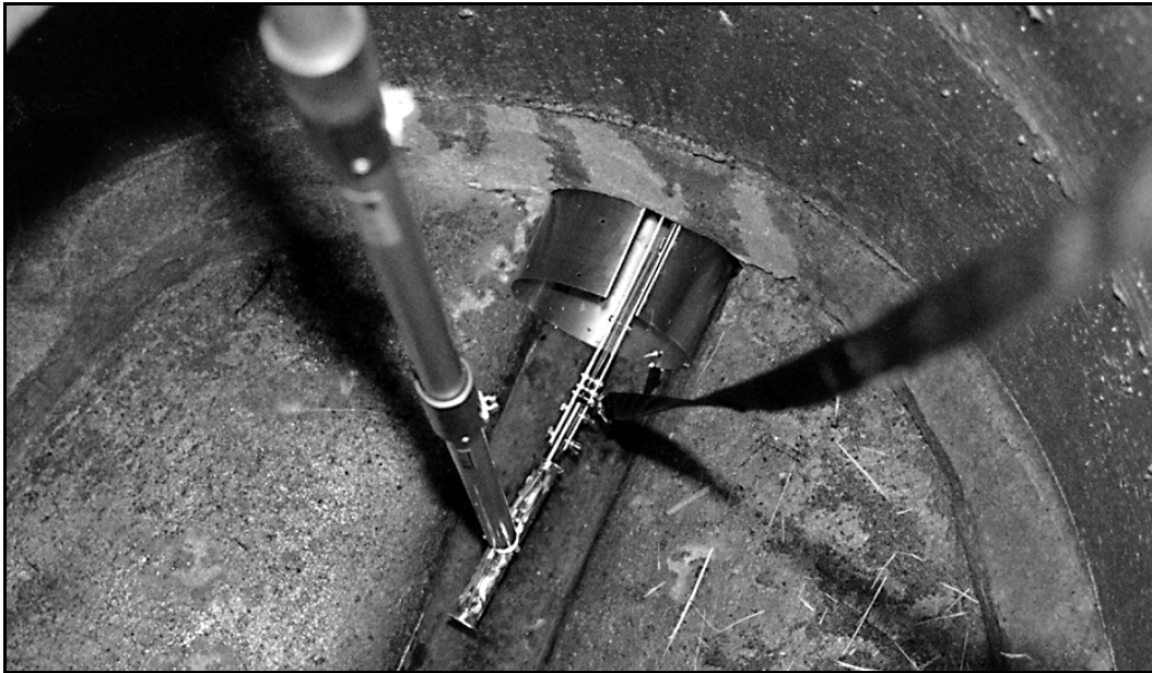
Figure 5-6 Inserting the Ring in the Upstream Channel
