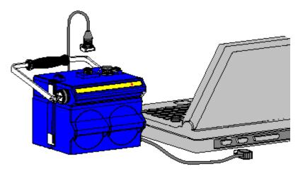
The 2101 Field Wizard does not have a case top connector. Instead, the communications cable attaches to the connector on the right side of the case.
