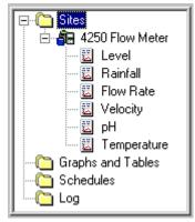
As you can see, the database now holds the site and instrument information, as well as downloaded readings such as Level, Rainfall, etc., contained in *Data Sets*.
