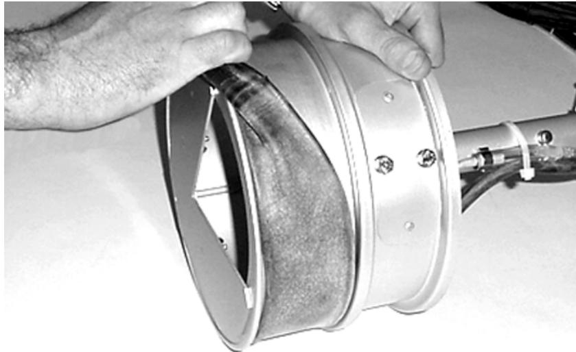
*Figure 3-1 Removing the Metering Insert's Rubber Collar*
