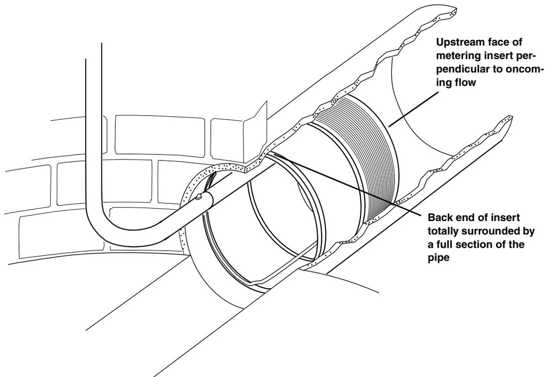
*Figure 2-9 Insert Installed in Sewer Pipe*
