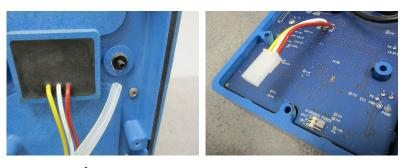
Figure 2-5 Disconnecting electrical connector and reference line
