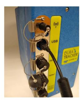
Figure 3-1 USB installation
