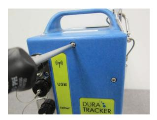
Figure 4-1 Screw removal
