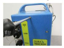
Figure 2-4 Screw removal
