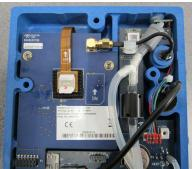
Figure 2-9 Installing SIM card
