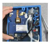
Figure 2-7 Plugging modem into circuit board
