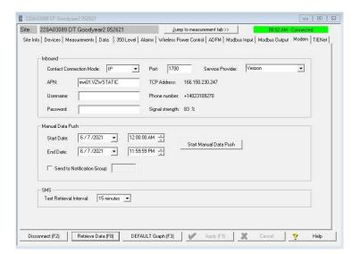
Figure 3-3 Flowlink Modem Tab
