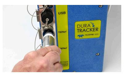
Figure 2-12 Connecting a TIENet sensor cable
