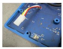
Figure 4-2 Disconnecting electrical connector and reference line
