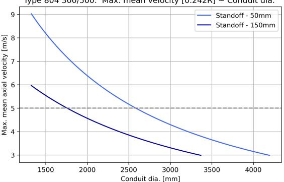
Type 804 300/500. Max. mean velocity [0.242R] ~ Conduit dia.
