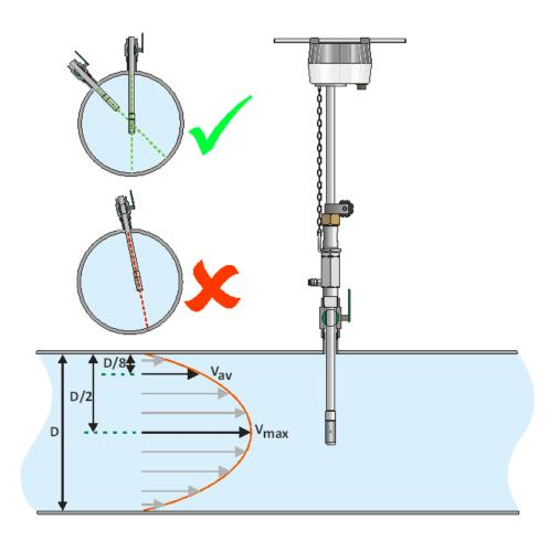
A transducer position at <sup>7</sup>/<sub>8</sub> pipe diameter can also be used if the clearance height above the pipe is an issue. The Configure App will compute insertion and profile factors for this position.
