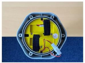
• Loosen the six screws around the lid using a 0.85Nm torque screwdriver.
