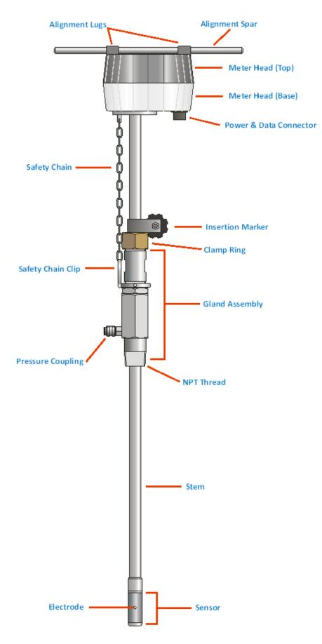
The device is available in two versions, differing in length to suit a wide range of pipe sizes. The precise dimensions of each version are discussed in Section 1.4. However, the various parts of each system are similar as described below:
