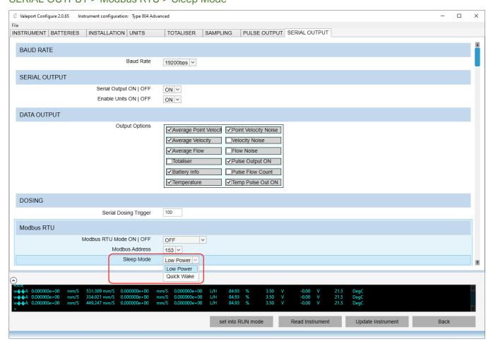
Quick Wake mode will keep the instrument in a raised power state which allows for a quick response to a Modbus command. This setting will have a large impact on the battery life of the Type 804. Use the battery life calculation to assess this.
