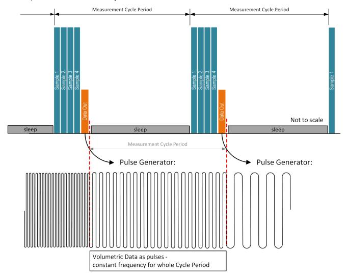
Look at the Pulse frequency from the 3 Measurement Cycle Periods in the diagram above — the flow is slowing down.
