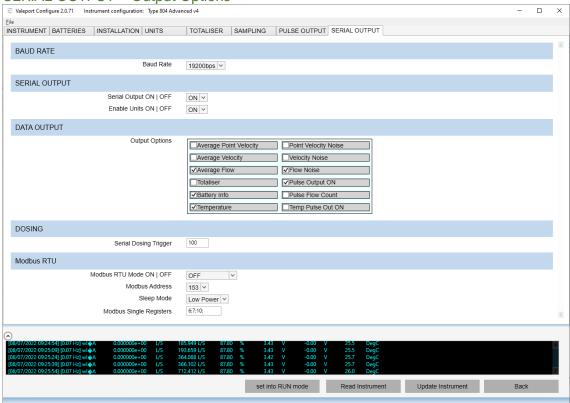
The serial string, seen in the terminal window across the bottom of the app, is made up of a standard set of fields followed by those selected in the form shown above:
