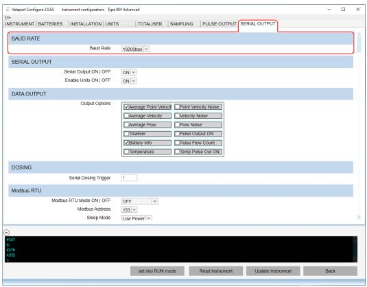
There is the option to use Modbus RTU over RS232 and RS485.
