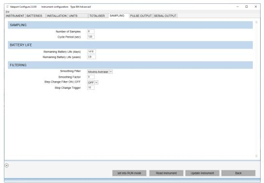
Measurement Cycle Period and Number of Samples are set using in the Configure App. They have a major effect on the battery life of the system. For this reason, the battery calculations are repeated on the Tab.
