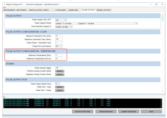
Select Temperature in the Output Options to switch on the output – both Pulse and Serial.
