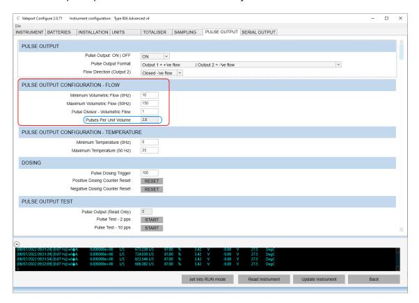
Follow a similar process if you intend to monitor Temperature in PULSE OUTPUT CONFIGURATION – TEMPERATURE
