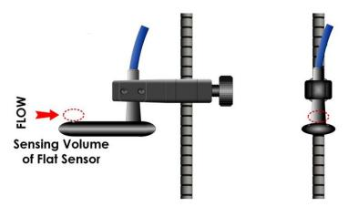
The sensor should be aligned into the flow, and the calibration is determined for +ve flow (flow on to the sensor at the electrode end) with the sensor upstream of the wading rod.
