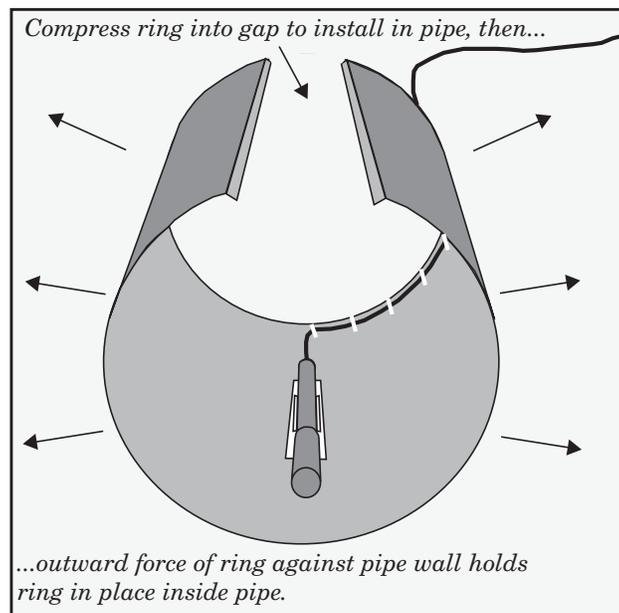
Figure 4-12 Sensor Installed on a Spring Ring
