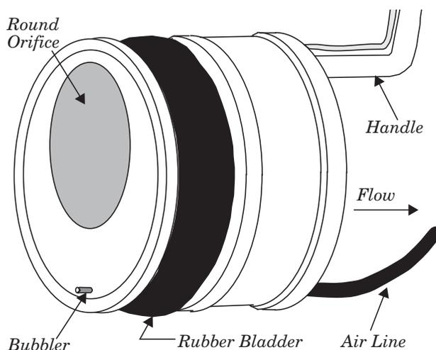
Figure 2-2 Flow Metering Insert
