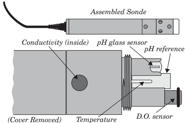
Figure 2-1 The YSI 600 Sonde
