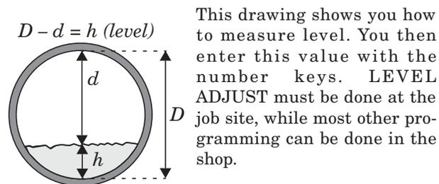
Figure 2-3 Level Measurement in Round Pipes
