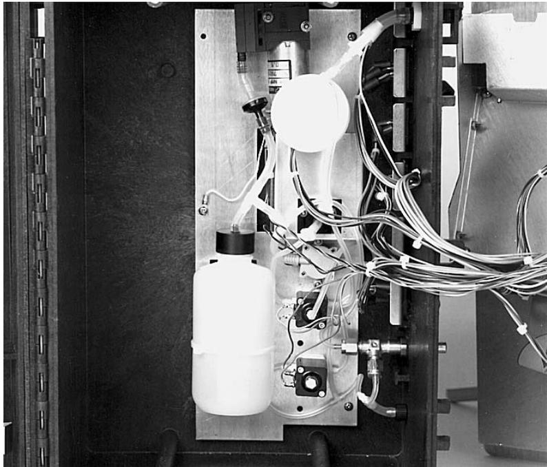
Figure 5-6 4230 Bubbler System Pressure Control
