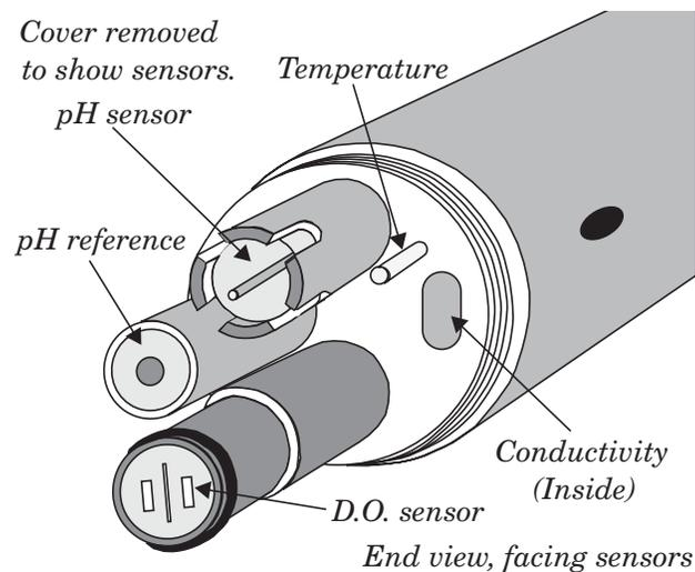
Figure 4-14 YSI 600 Multiple Sensor Sonde
