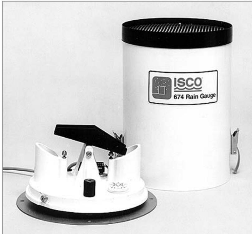
Figure 4-6 674 Tipping Bucket Rain Gauge
