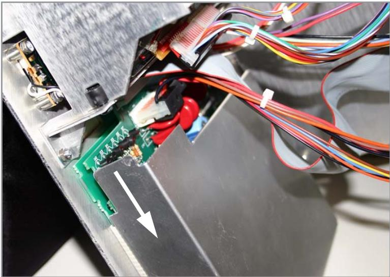
Figure 4-4 Removing the lower shield
