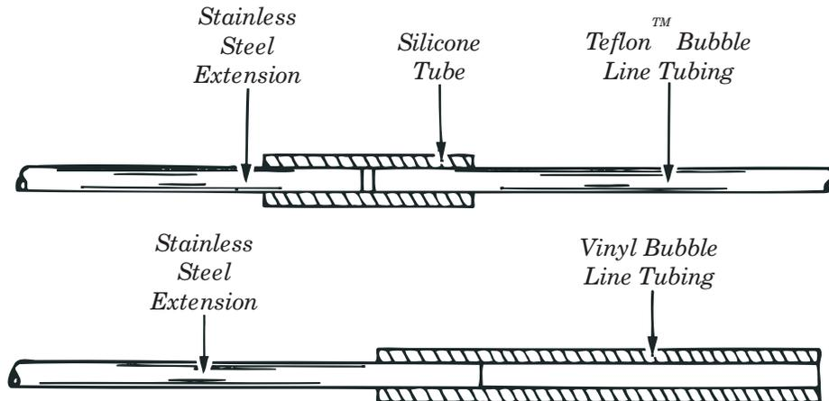
Figure 3-5 Installing the Stainless Steel Bubble Line Extension
