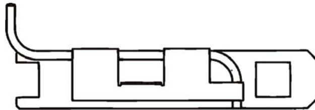
Figure 3-7 Bubbler Tube Retainer Assembly
