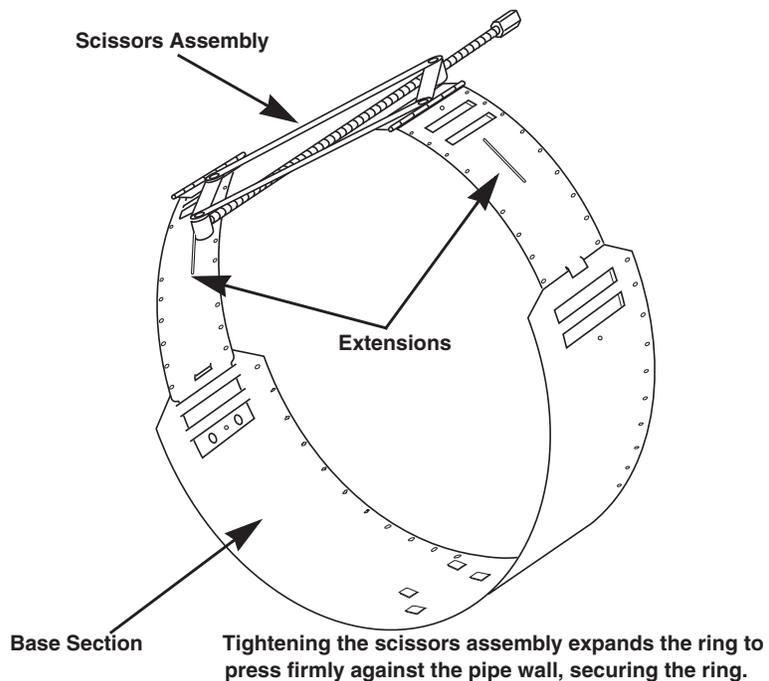
Figure 4-13 Scissors Ring Adjustment
