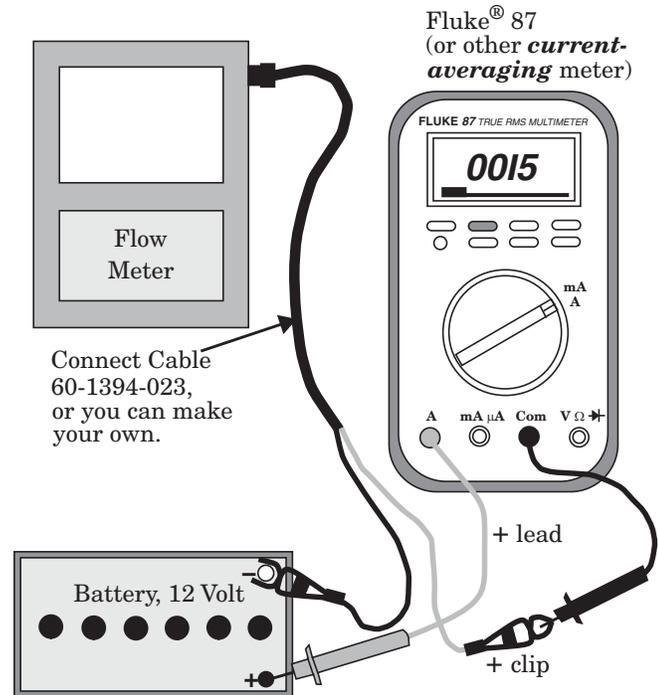
A good quality, adjustable, regulated DC power supply can be substituted for the 12-volt battery. The power supply should have at least 3 Amperes output, preferably more, and capable of overcurrent surges.
