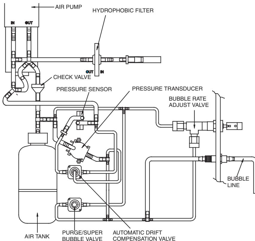
Figure 5-7 Schematic Diagram of the Bubbler System
