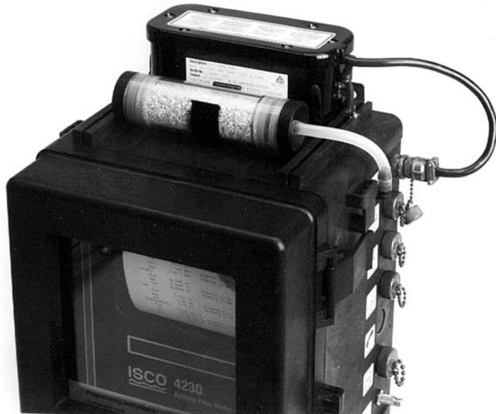
Figure 3-1 Battery Installed on Flow Meter
