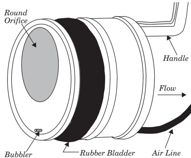
Figure 3-6 Flow Metering Insert
