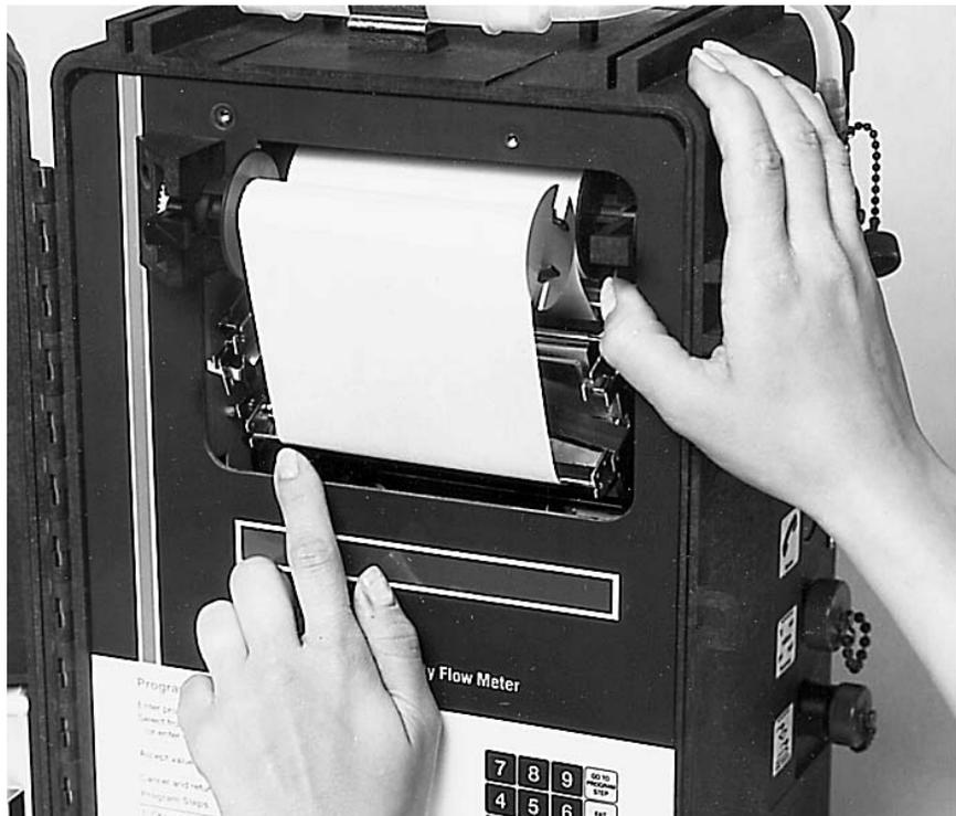
Figure 5-4 Lifting the Flow Meter from the Case
