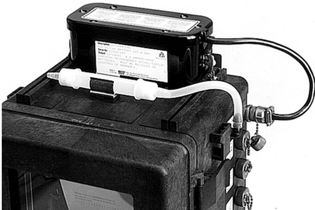
Figure 3-1 Nickel-Cadmium Battery Installed on a Flow Meter
