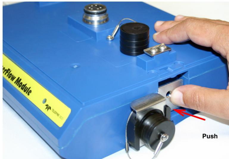
*Figure 1-4 Unlocking the latch*
